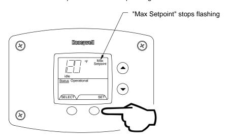
Step 5: 30 Seconds after the last button press, the Water Heater Display will go back to "User Mode". It will read "Max Setpoint" without showing a temperature value if the temperature setpoint is at the maximum setting. The Water Heater Display can be set back to the "User Mode" immediately by pressing both the "Temperature Up" and "Select" buttons together for 3 seconds.
